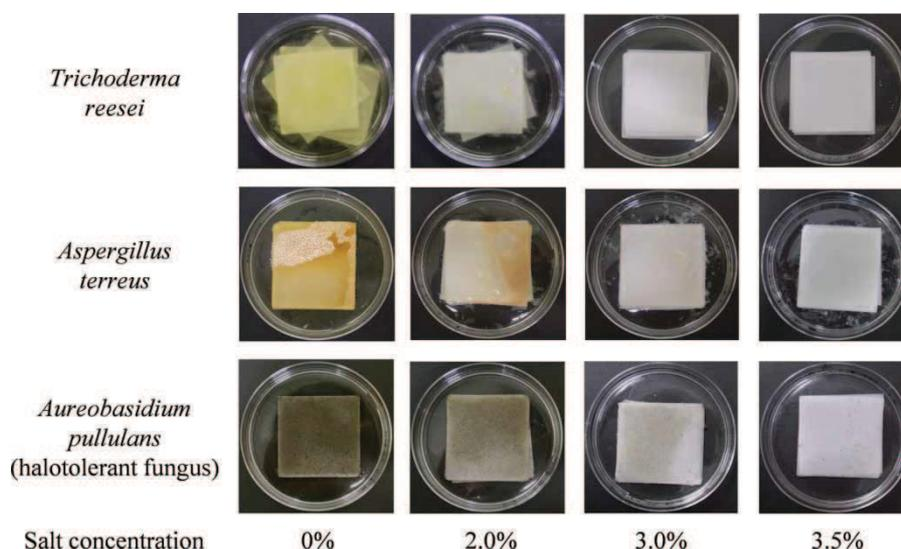
Figure 5 Photographs of copy paper samples at varied salt concentrations seven days after inoculation with fungal spores.
