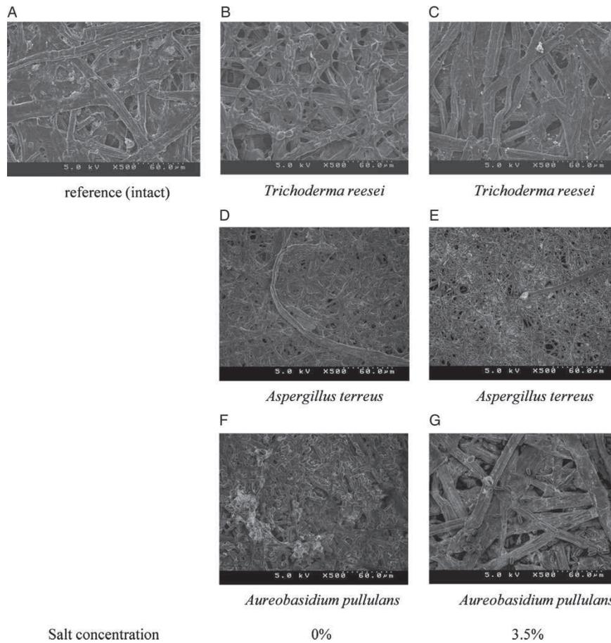
**Figure 6** SEM images of copy paper: (A) intact copy paper; (B) and (C) *T. reesei*; (D) and (E) *A. terreus* at 0 and 3.5% salt concentration, respectively and (F) and (G) *A. pullulans* at 0 and 3.5% salt concentration, respectively.
